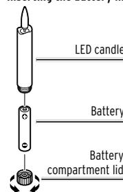
1. Remove the lid of the battery compartment of the candle by turning it anti-clockwise.
